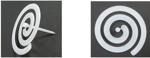
**Fig. 8** Spiral flow specimen
