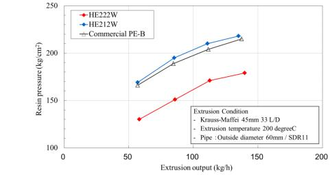
Fig. 7 Processability data-2: relationship between output and material pressure
