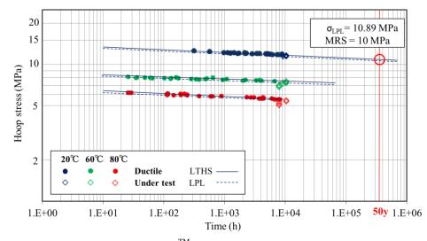
Fig. 5 Hydrostatic strength data of NOVATEC<sup>TM</sup> HD HE222W : determined at EXOVA
