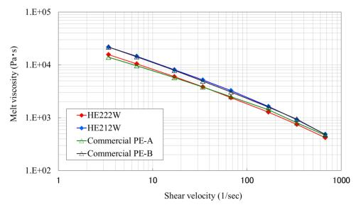
Fig. 4 Shear rate dependence of viscosity at 190 degree C
