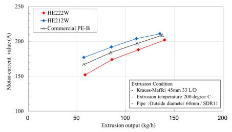
Fig. 6 Processability data-1: relationship between output and motor-current
