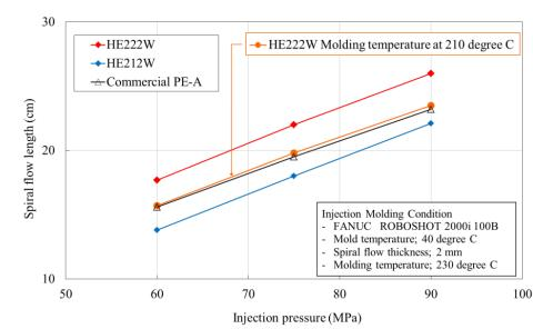
Fig. 9 Processability data-3: relationship between injection pressure and spiral flow length
