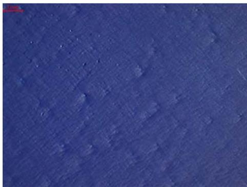
**Fig. 2** The inner wall of the pipe made from the material which has a poor dispersion of HMWC
